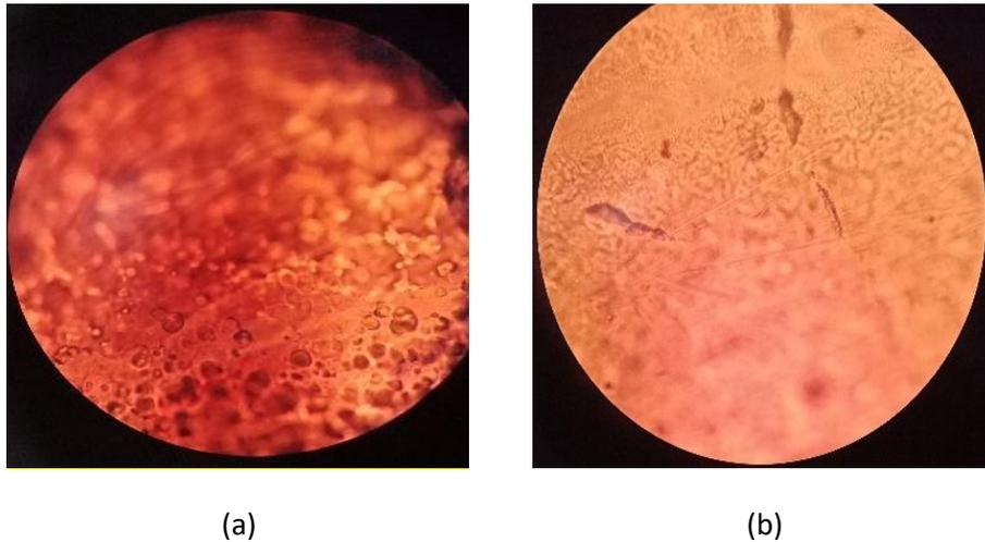
Fig. 2. Images of the samples at magnification of 100x: (a) CCH9:1 stirring at room temperature and (b) CCH9:1 stirring at 80°C
