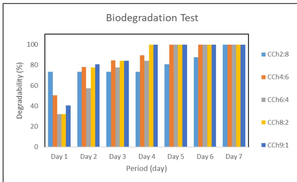
Fig. 3. Biodegradability of the samples of: (a) CCH2:8; (b) CCH4:6; (c) CCH6:4; (d) CCH6:4; (e) CCH8:2 and (e) CCH9:1
