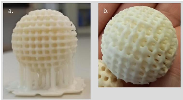
Fig. 2. The 3-D printed sphere nanocomposite incorporated with TiO<sub>2</sub>. (a) Before treatment; (b) After treatment.
