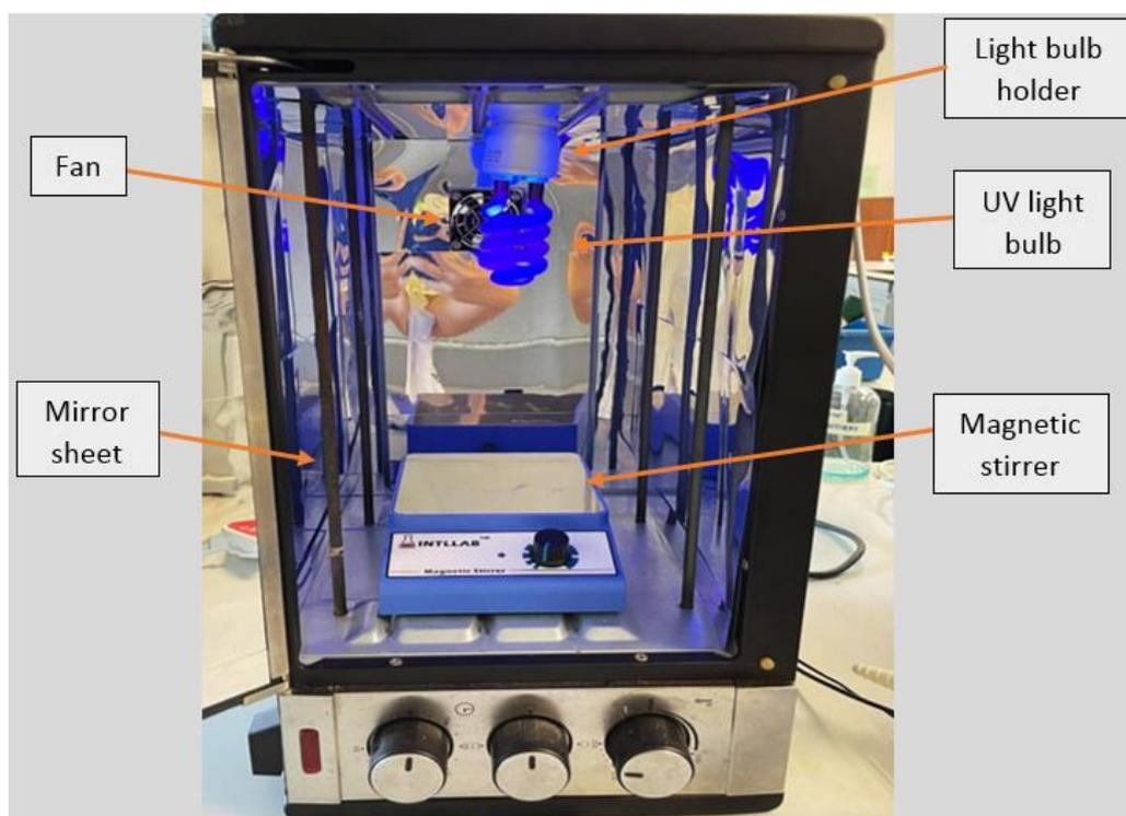
Fig. 4. Design of a low-cost photoreactor equipped with UV light.
