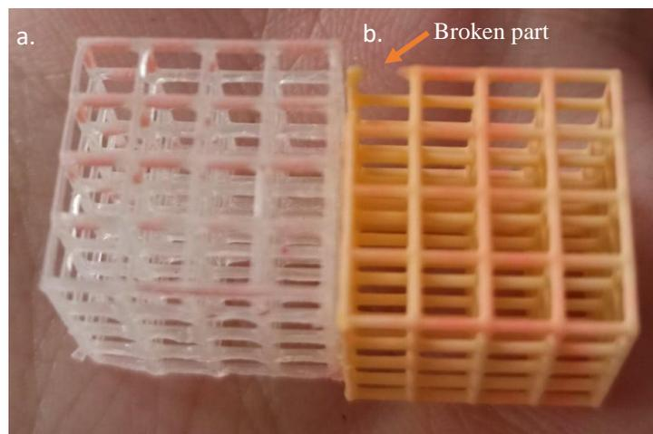
Fig. 3. The cubic structures: (a) before magnetic stirring (b) after treatment magnetic stirring.
