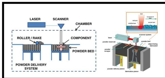
Fig. 1. Working principle of Selective Laser Melting (SLM) (Prashanth, 2020).
