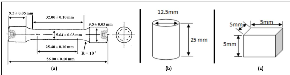
Fig. 2. (a) Tensile Test Specimen (b) Compressive Test Specimen (c) Hardness Test Specimen (Pelleg, J. 2012).
