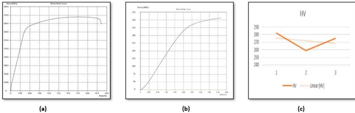
Fig. 3. (a) Tensile Test Result (b) Compressive Test Result (c) Hardness Test Result
